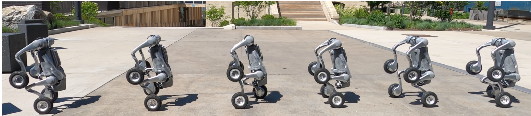
Figure 3: Sim-to-Real Deployment. We successfully deploy a two-legged handstand walking policy, generated via MimicAgent, directly onto the Go2-W quadruped. Despite being trained entirely in simulation, the policy achieves a stable forward walking gait at 0.4 m/s. See the supplementary material for full details regarding sim-to-real transfer and hardware deployment.
